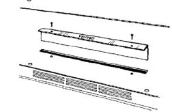
■ Turn vent baffle and reinsert in slot in top of range hood so that the word 'Vented" is facing up. Fasten vent baffle with screws.
